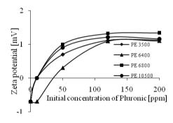
Fig. 12. Zeta potential of magnesite in the presence of Pluronics as a function of copolymer concentration (C<sub>NaCl</sub>= 1·10<sup>-4</sup> M, pH 8.5)
