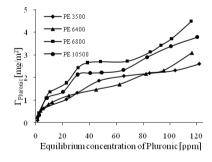
Fig. 2. Adsorption isotherms of Pluronics on dolomite (pH 10.4 and  $C_{NaCl}$ =1·10<sup>-4</sup>M)
