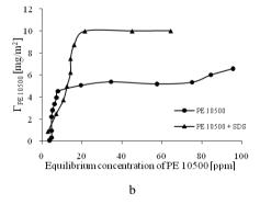
Fig. 10. Adsorption isotherms of Pluronic PE 6800 (a) and PE 10500 (b) on magnesite from the mixed solution (SDS concentration - 120 ppm,  $C_{NaCl}$ =1·10<sup>-4</sup>M, pH 8.5)
