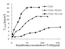
Fig. 4. Cationic surfactant adsorption on dolomite from mixed solutions (Pluronic concentration - 120 ppm, pH 10.4,  $C_{NaCl} = 1 \cdot 10^{-4} \text{ M}$ )
