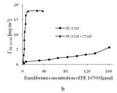
Fig. 7. Adsorption isotherms of Pluronic PE 6800 (a) and PE 10500 (b) on dolomite from mixed solution (CTAB concentration - 120 ppm,  $C_{NaCl}$ =1·10<sup>-4</sup>M, pH 10.4)
