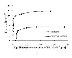
Fig. 6. Adsorption isotherms of Pluronic PE 6800 (a) and PE 10500 (b) on magnesite from mixed solution (CTAB concentration - 120 ppm,  $C_{\text{NaCl}}$ =1·10<sup>-4</sup>M, pH 8.5)
