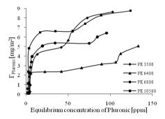
Fig. 1. Adsorption isotherms of Pluronics on magnesite (pH 8.5 and  $C_{NaCl}$ =1·10<sup>-4</sup>M)
