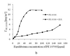
Fig. 11. Adsorption isotherms of Pluronic PE 6800 (a) and PE 10500 (b) on dolomite from the mixed solution (SDS concentration - 120 ppm,  $C_{NaCl}$ =1·10<sup>-4</sup>M, pH 10.4)
