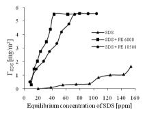
Fig. 8. Anionic surfactant adsorption isotherms onto magnesite from mixed solution from Pluronic-SDS solutions (Pluronic concentration - 120ppm, C<sub>NaCl</sub>=1·10<sup>-4</sup>M, pH 8.5)
