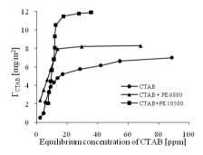
Fig. 3. Cationic surfactant adsorption on magnesite from mixed solutions (Pluronic concentration - 120 ppm, pH 8.5,  $C_{NaCl} = 1 \cdot 10^{-4} \text{ M}$ )
