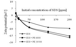
Fig. 16. Zeta potential of magnesite in Pluronic-SDS mixed solution as a function of anionic surfactant concentration (Pluronic concentration – 120 ppm, C<sub>NaCl</sub>= 1·10<sup>-4</sup> M, pH 8.5)
